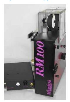
The RM100 is used for circumferential markings of cables wires, or cords using the proven hot stamping process. Foil coated on one side with printing substance is pressed onto the material with a hot stamp. Through pressure and heat the stamp is marked onto the material. In order to obtain a circumferential marking, two half-shells are used.
